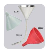
MARS No. 93398 Utility Funnel with Screen is the most popular allpurpose fluid dispenser. Galvanized steel. Includes screen and 12" flexible extension with tapered tip. Tip 4/16" OD / 9/16" ID.
