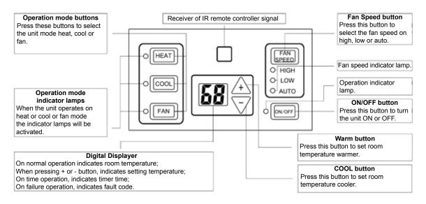
Fig. 12 Use of unit mounted control panel
