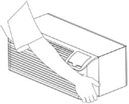
Fig. 6 Cabinet Front Removal View 1
