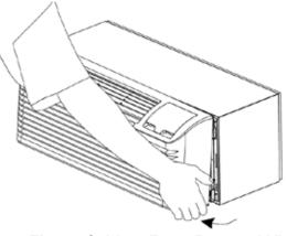
Fig. 7 Cabinet Front Removal View 2
